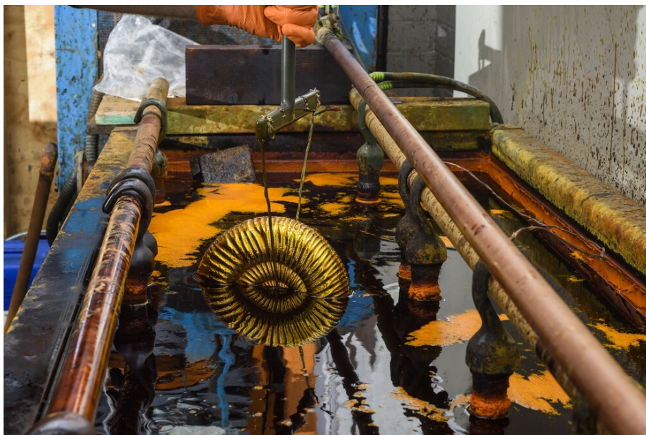
Fig. 17 Chrome-plating aluminium ammonite casts for Starship (Super Heavy) and Dry Cask (Silk Cut) , by Alice Channer. 2023. (Courtesy the artist and Konrad Fischer Galerie, Berlin; photograph Thierry Bal).
